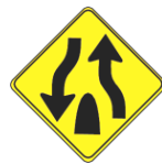
Divided Highway Ends
