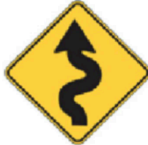
Winding road ahead.
